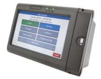
Incorporate employee ID badges for bar code or magnetic strip swipes. Biometric hand scanners confirm employee identity before allowing clock in/ out. Prevents co-workers from clocking in or out for one another.
